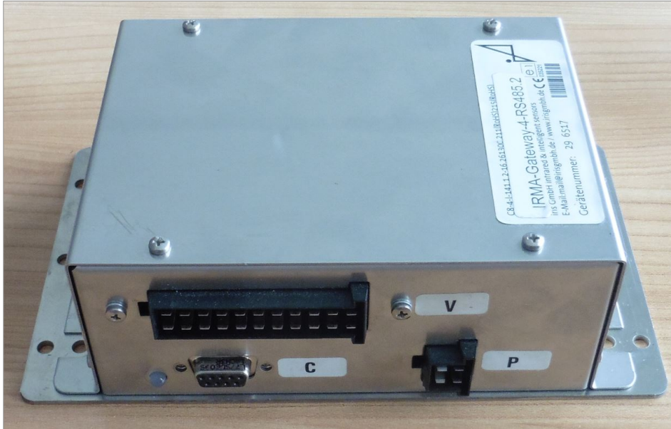
Fig. 2: View of IRMA-Gateway-4-RS485.2: operating interfaces and name plate
