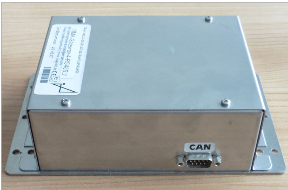
Fig. 3: View of IRMA-Gateway-4-RS485.2: sensor connection
